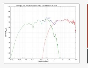
Extended response from 65 Hz to 18.5 kHz with efficient LF-HF crossover transition for impactful delivery.
