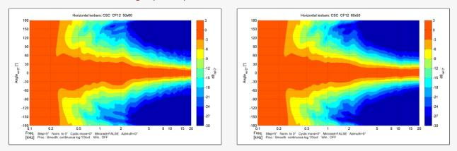
Narrow and smooth horizontal coverage from 500onwards with an average 60 degrees dispersion up to 10KHz.
