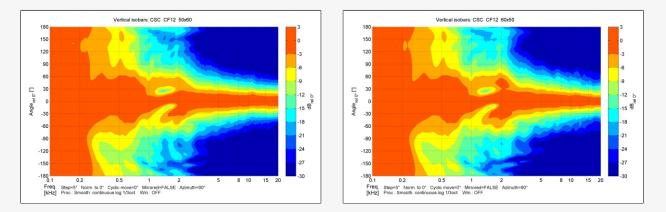
Maintains precise 50-degreevertical control from 1000 Hz onwards.
