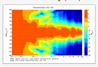
Stable 90° horizontal coverage makes CC8 ideal for distributed audio systems. Even dispersion minimizes overlaps in ceiling or wall-mount grid configurations.
