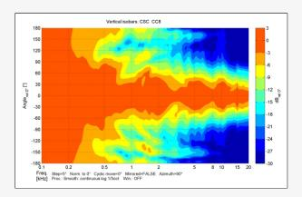
The CC8's compact coaxial design maintains balanced vertical dispersion of 90° across short-throw distances. Its consistent beam control ensures clear coverage in smaller venues or nearfield applications.
