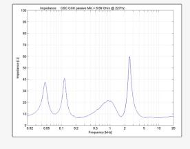
Maintains nominal 8-ohm load with predictable impedance profile, simplifying amplifier matching and ensuring a stable installation.
