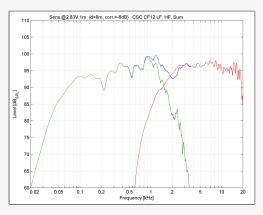
Extended response from 65 Hz to 18.5 kHz with efficient LF-HF crossover transition for impactful delivery.
