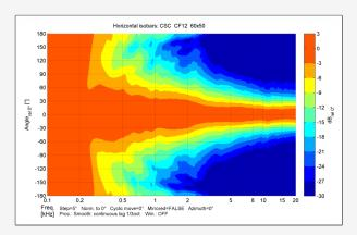
Narrow and smooth horizontal coverage from 500 Hz onwards with an average 60 degrees dispersion up to 10 KHz.
