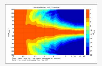
Narrow and smooth horizontal coverage from 500onwards with an average 60 degrees dispersion up to 10KHz.
