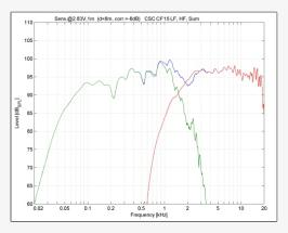
Extended response from 60 Hz to 18.5 kHz with efficient LF-HF crossover transition for impactful delivery.
