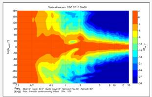
Maintains precise 50-degreevertical control from 1000 Hz onwards.
