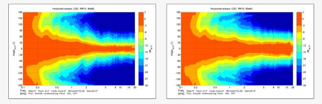
Maintaininga uniform vertical dispersion of 60 degrees right up to 15k. The vertical isobars show a smooth transition as the frequency increases from 500hz to 17Khz.
