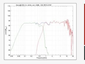
With a smooth response, it has a frequency response from 65 Hz to 18.5 kHz. Designed for full-range clarity or integration with a bass cabinet.
