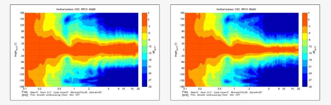
Designed for medium-throw use, the RR15 maintains uniform vertical dispersion of 40 degrees rightup to 15k. The vertical isobars show a smooth transition as the frequency increases from 500hz to 16 Khz.
