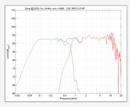
With a smooth response, it has a frequency response from 65 Hz to 18.5 kHz. Designed for full-range clarity or integration with a bass cabinet.
