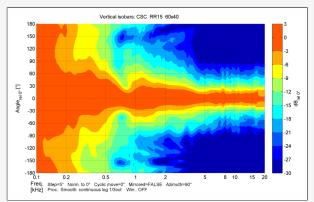
Designed for medium-throw use, the RR 15h maintains uniform vertical dispersion of 40 degrees right up to 15 kHz. The vertical isobars show a smooth transition as the frequency increases from 500hz to 16 Khz.
