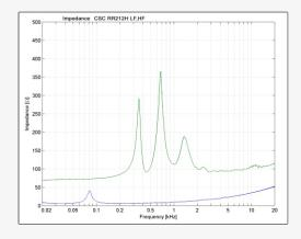
The Nominal 4-ohm impedance for both LF and HF section simplifies amplifier selection.
