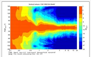
Designed for medium-throw use, the RR 212hdespite its MTM design maintains uniform vertical dispersion of 40 degrees. The vertical isobars show a smooth transition as the frequency increases from 500hz to 16 KHz.
