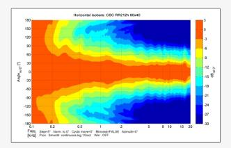
With its smooth and uniform Horizontal dispersion of 60 degrees, it shows a smooth transition as the frequency increases from 500hz to 16 KHz.
