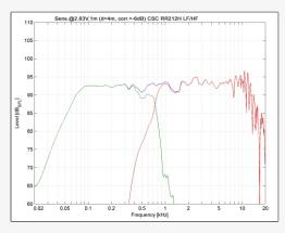
Covers 65 Hz to 17.5 kHz cleanly, designed for full range deployment.
