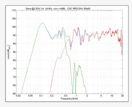
The 3-way system is crossed passive/active crossover topology achieves a smooth response from 70 Hz to 20 kHz.
