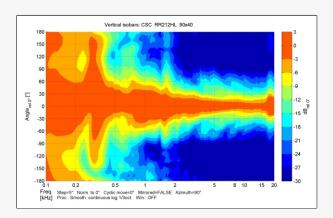
Designed for array configurations, the RR 212hl-40, RR212HL-60 and RR212HL-90 maintaina highly controlled vertical dispersion of 40°, enable tailored vertical coverage in flown or stacked deployments.
