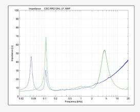
Maintains dual 8-ohm impedance LF and HMF. These plots aid amplifier matching and system protection in high-power installations where speaker arrays present complex loads.
