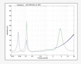
Maintains dual 8-ohm impedance LF and HMF. These plots aid amplifier matching and system protection in high-power installations where speaker arrays present complex loads.
