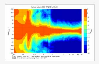
Designed for array configurations, the RR 212hl-40, RR212HL-60 and RR212HL-90 maintaina highly controlled vertical dispersion of 40°, enable tailored vertical coverage in flown or stacked deployments.
