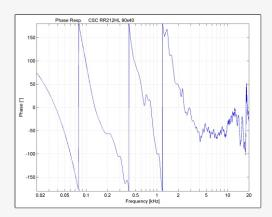
With a minus 50-degree phase angle between 2kHz and 20kHz it ensures accurate midrange propagation. This performance ensures intelligible vocals and instruments in complex acoustic spaces like stadiums or cathedrals.
