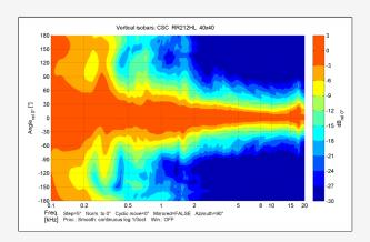
Designed for array configurations, the RR 212hl-40 MK1, RR 212hl-60 MK1 and RR 212hl-90 MK1 maintain a highly controlled vertical dispersion of 40°, enable tailored vertical coverage in flown or stacked deployments.
