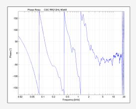
With a minus 50-degree phase angle between 2kHz and 20kHz it ensures accurate midrange propagation. This performance ensures intelligible vocals and instruments in complex acoustic spaces like stadiums or cathedrals.
