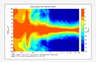
Designed for array configurations, the RR 212hl-40 MK1, RR 212hl-60 MK1 and RR 212hl-90 MK1 maintain a highly controlled vertical dispersion of 40°, enable tailored vertical coverage in flown or stacked deployments.
