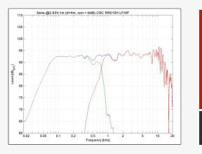
Extended response from 65 Hz to 18.5 kHz with efficient LF-HF crossover transition.
