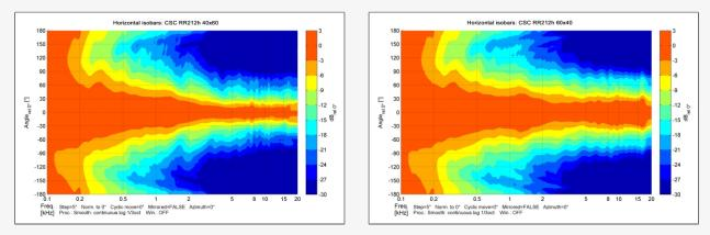
A smooth and consistent horizontal coverage from 500 onwards with an average 60 degrees dispersion for intelligible audio.
