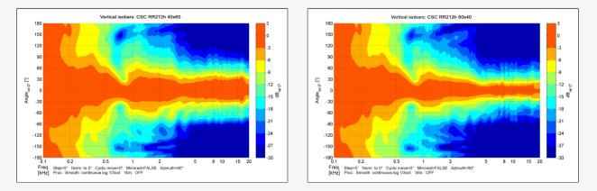
Maintains precise and smooth 45-degreevertical control upto10KHz.
