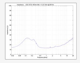
16 ohms nominal with low inductance design for smoother frequency response and amplifier ease.
