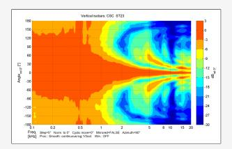
The ST23's dual 3" wideband drivers ensure tight vertical beam control of plus minus 40 degrees up to 8 kHz, reducing ceiling/floor reflections in compact zones.
