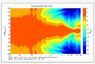
Delivers 90° horizontal spread up to about 7 kHz making it suitable for most vocal applications.
