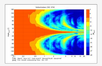
ST43's cabinet design for extremely narrow vertical dispersion. It offers a 20-degreevertical dispersion up to 6 kHz.
