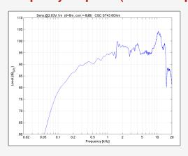
Response from 150 Hz to 16 kHz makes it suitable as a standalone or with a subwoofer.
